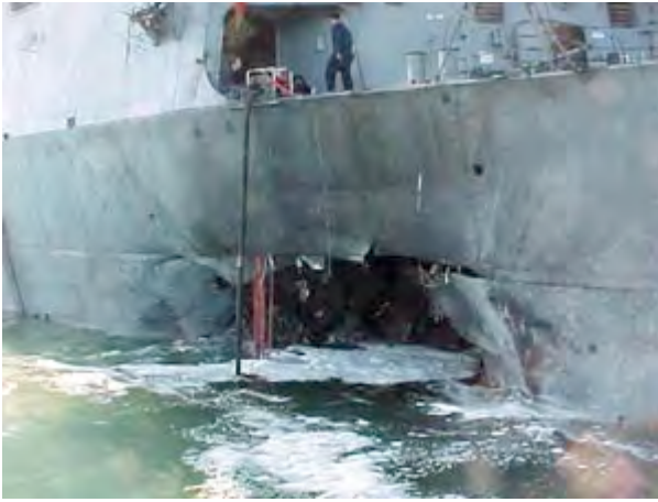
Figure 2: Damage to the Cole .
